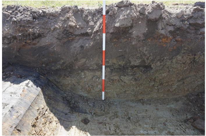
Plate 35: Looking south west at section exposed in test pit 6 located at NW end of the trench 6. Victorian top soil horizon is a thin black band behind second from the base white section of the scale. Context below buried topsoil is alluvium and context above are made ground levelling deposits (603 and 604) followed by railway bedding (602) sealed by demolition deposit (601)
